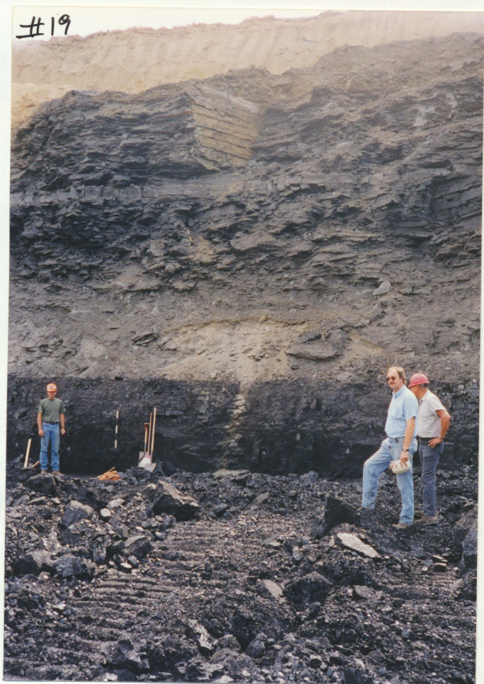
Razorback Mine, 6/16/99 Pit showing coal and overlying strata at sampling site. Note gray shale directly above coal (Energy sh.), ~10ft, then Anna sh. & Brecken 25.
