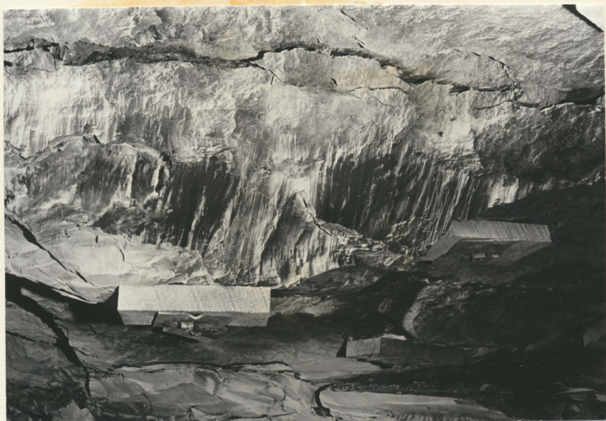
Closeup showing highly polished and slickensided surface of same slip fracture.
