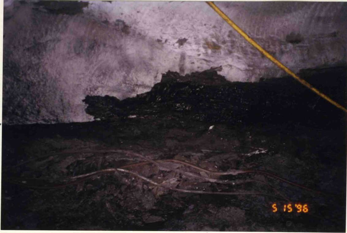
A. Photo taken looking northwest, probably near station 1 on map. The top and bottom of the coal have been sheared are bounded by shear planes. The roof sediments, coal, and floor have been distorted and contain flow features and microfaulting and thrusting.
