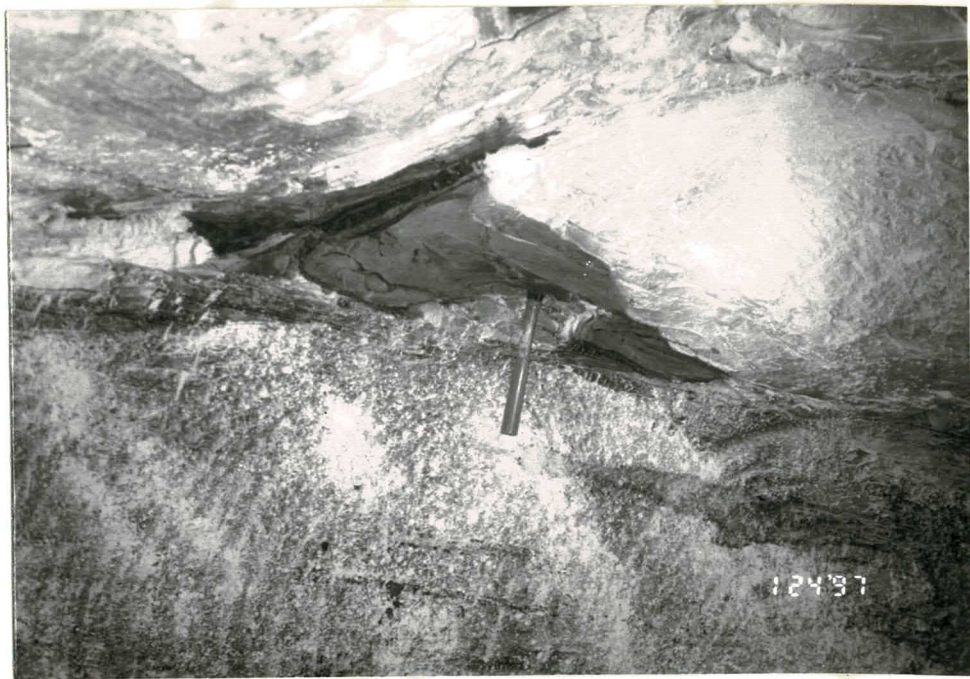
A large roll. Location #11, Riola Mine
