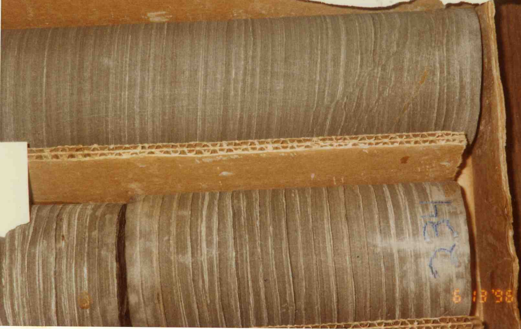
Close-up of micro slumping in core from Catlin Coal Co. hole #2
