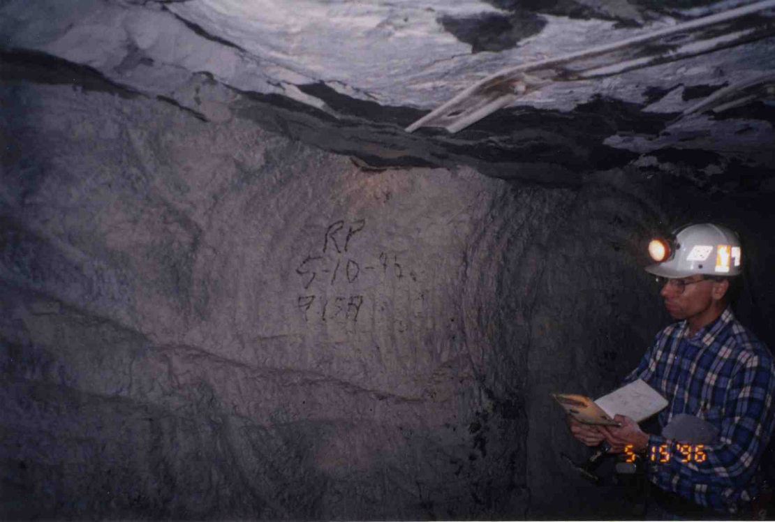
photo was probably taken near station 6. Rida Mine seam is nearly full height. Disturbed roof, including possible liquifaction f exposed above the coal. Colin Treworgy holds the notebook.
