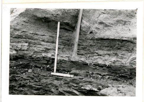
Closeup view with pick point imbedded in gray clay layer. Black shale below clay band, and coarse, loose sandstone above.
