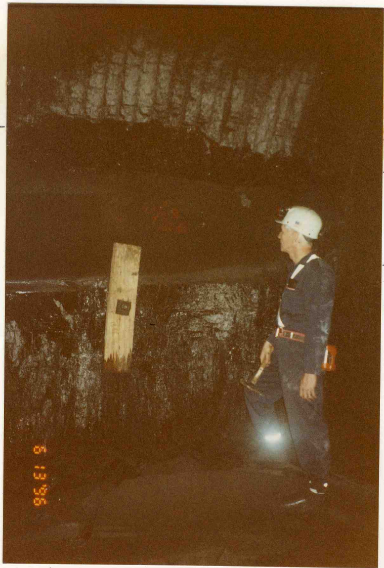
Marvin Thompson examines a large parting in the Springfield Coal. The roof bolt had been installed in the rib to prevent the parting from falling. This did not work - about 1 foot of the
