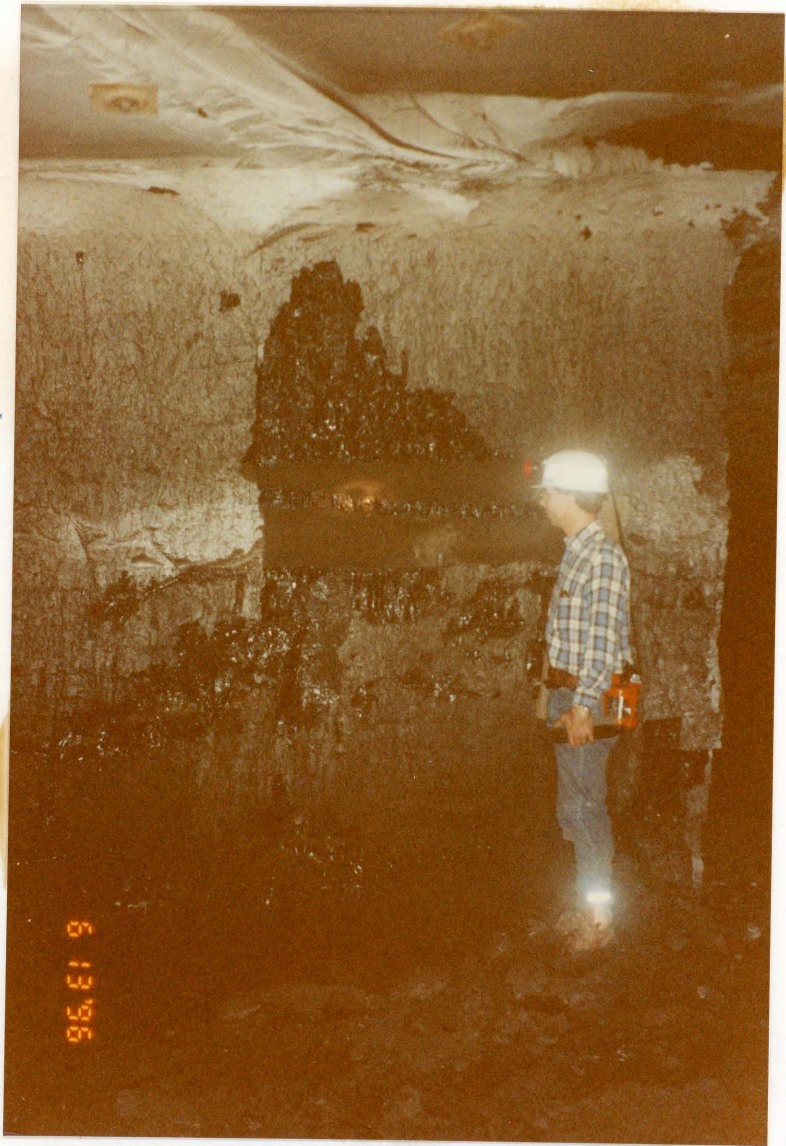
Colin Treworgy (5'9") stands by the Springfield coal (about 9 feet thick) examining a parting.
