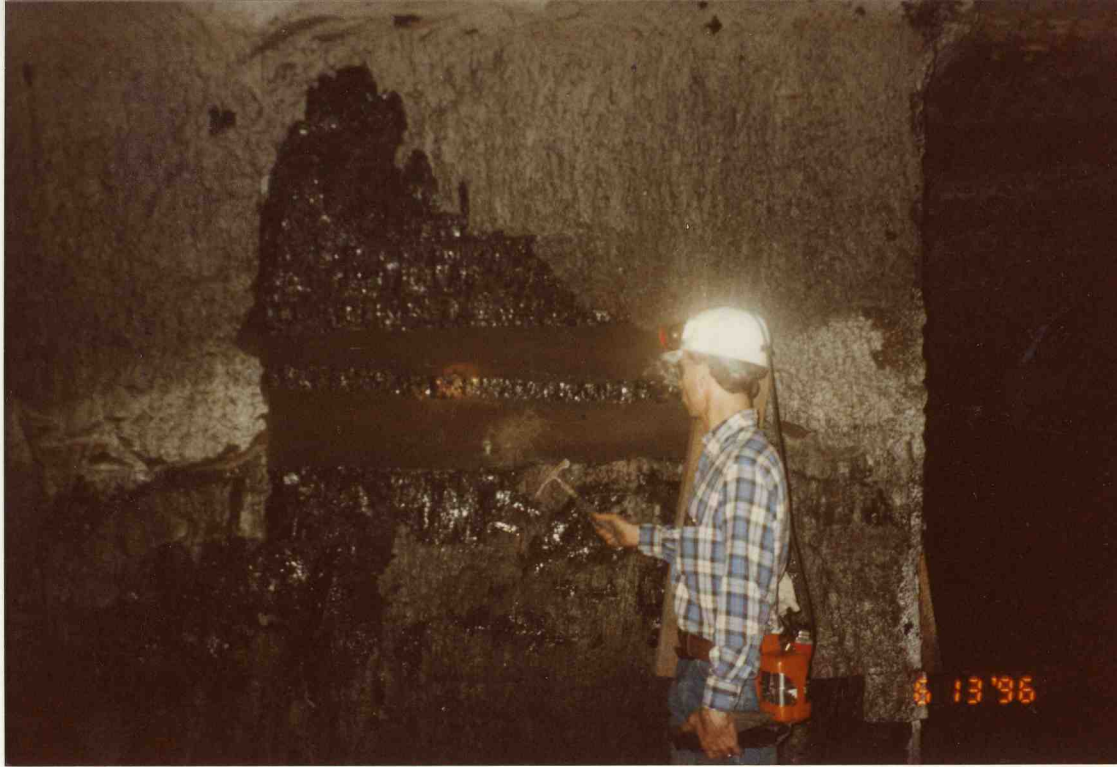
Colin Trewoogy examines a parting in the Springfield Coal, Wabash Mine. Note the thin bench of coal within the parting. The parting is continuous to the left and right, but has been obscured by rock dust
