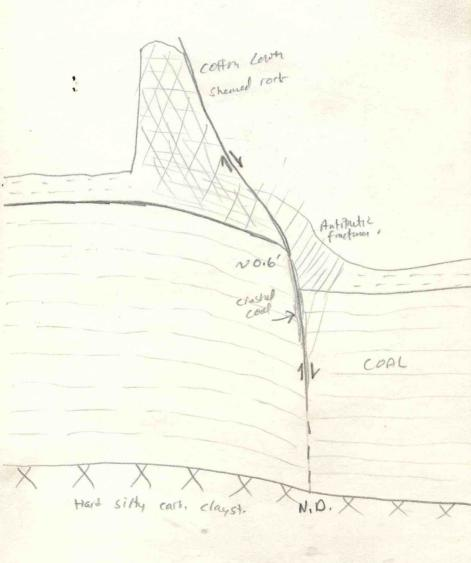
ing fractures NE of the fault and several low-angle to horizontal shears SW of the fault, with slickensides trending 085.
