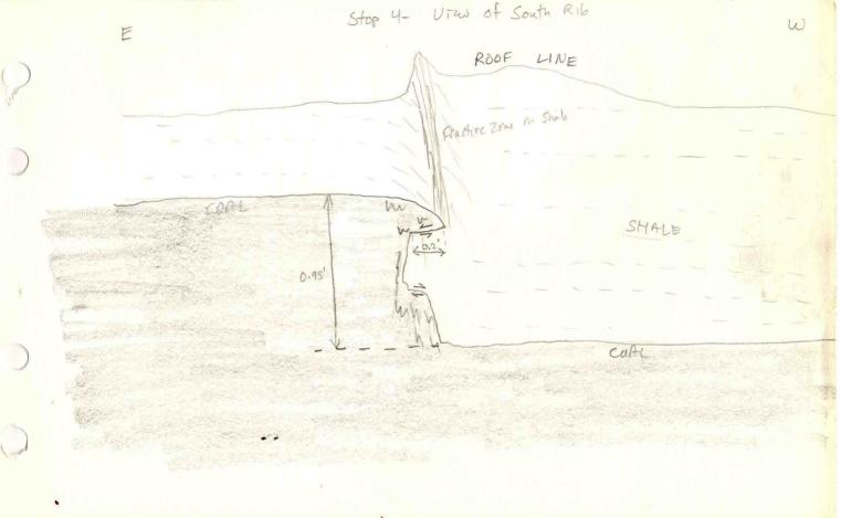
8. Fault on south rib (photo) does not show a single clean break, but the coal is closely fractured and dragged downward along a set of downward-fanning fractures. Displacement decreases to north and the feature becomes a clean fault. This structure not noted in track entry.
