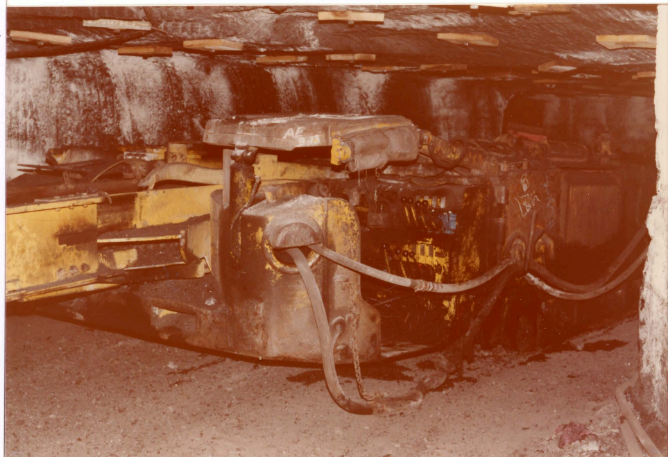
Operator's control position for continuous miner.
