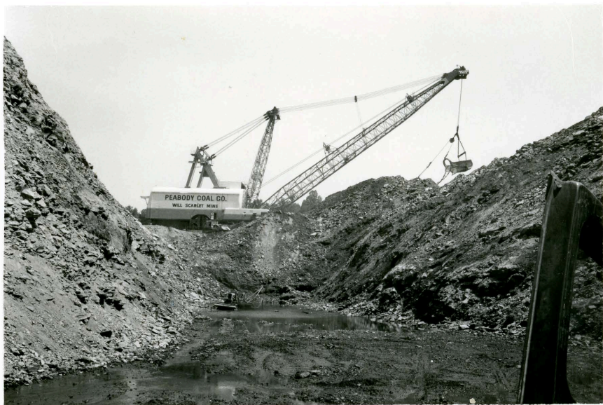
Dragline removing overburden at east end of pit (Stop 1). Steep loose highwall to left and partially covered highwall to right (east).
