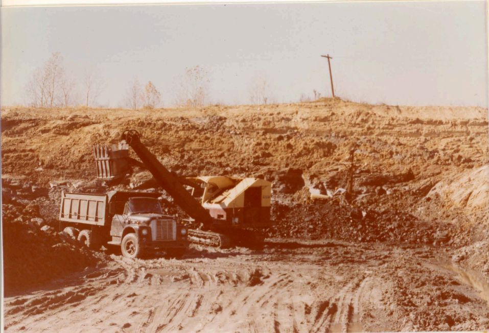
Small shovel loading Harrisburg (No. 5) Coal into dump truck at Crenshaw Coal Co. No. 1 Mine. Highwall in background includes about 10 feet of gray shale overlain by glacial drift. Photo by. J.N., 11/9/78.
