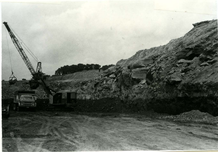
General view of the operations at Big Ridge Coal Co. strip pit. The dragline in the background is removing the overburden while the shovel loads coal into dump trucks. Photo by Heinz Damberger, 5/30/74.
