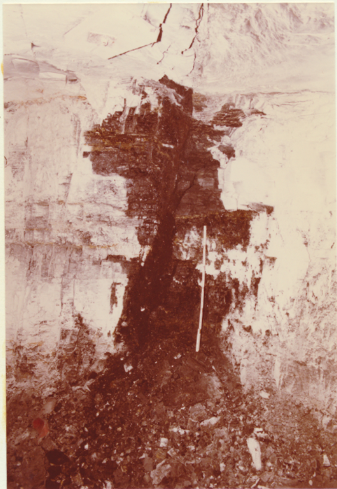
Fault on travelway of 8th Panel South. Coal is up-thrown 2.7 feet on the southeast (left) side of the fault. Coal is folded and pulverized along the surface of movement.
