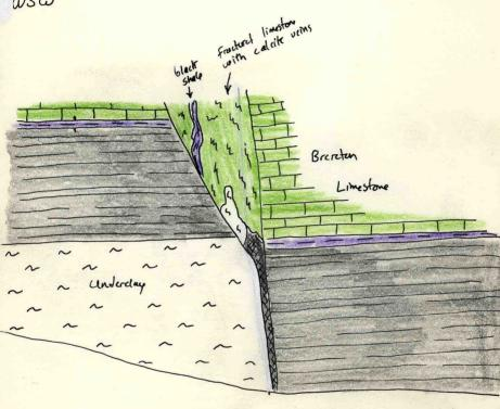
At first glance a simple normal fault, branching upward; but note underclay squeezed upward along fault plane.
