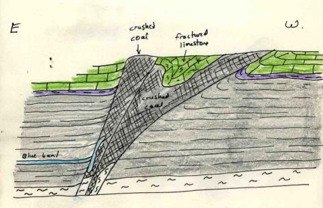
Almost no net displacement across fault, but fault sixes show both normal and reverse offset.
