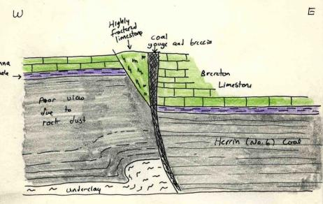
The main offset is a normal fault, but note the reverse flexure in the floor on the footwall, and the coal gouge along the fault above the position of the Herrin coal on either side of the fault.
